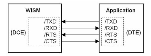
Port /RXD of the WISM transmits data to the application's /RXD input.
